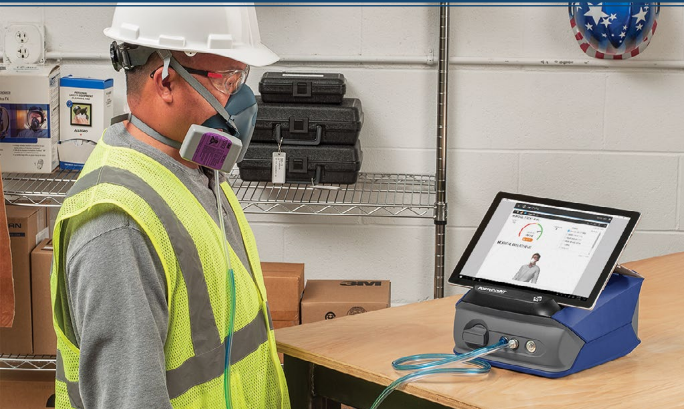
The PortaCount® Respirator Fit Tester measures the concentration of ambient particles outside the respirator and the concentration of ambient particles inside of the respirator. (photo courtesy TSI)
