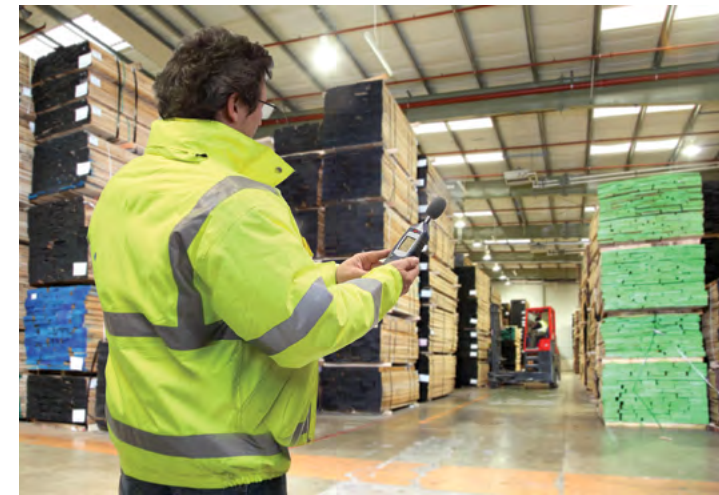
To ensure adherence to OSHA regulations, monitoring provides accurate insights into the noise levels of a working environment, identifying where the problem areas are. (photo courtesy Casella)
