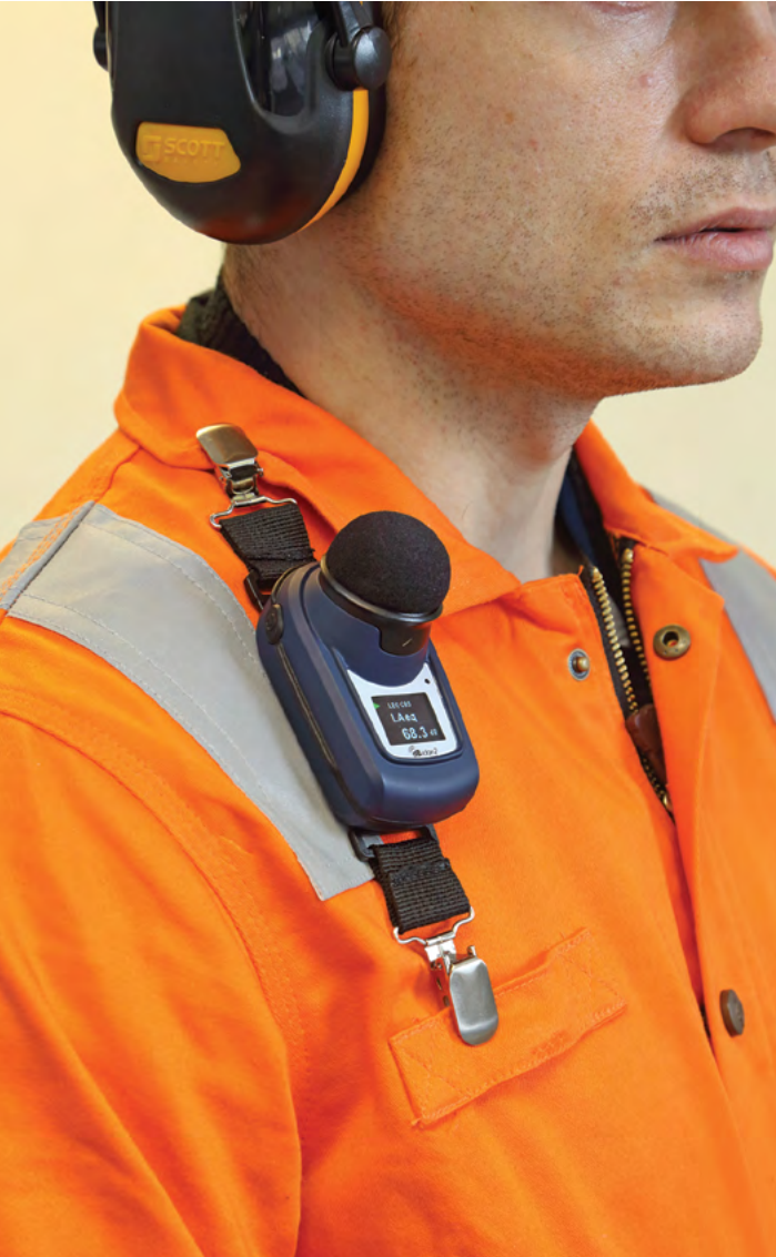
Noise dosimeters are small, body-mounted devices that collect individual exposure data, typically worn during an employee's entire shift. (photo courtesy Casella)
