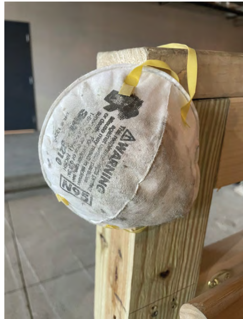
Case studies show the annual total cost of ownership (per wearer) for a disposable N95 mask is high compared to the cost of re-usable, half-face air-purifying respirators fitted with HEPA cartridges. (photo courtesy DPS Group)
