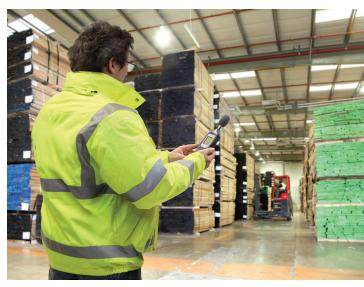
To ensure adherence to OSHA regulations, monitoring provides accurate insights into the noise levels of a working environment, identifying where the problem areas are. (photo courtesy Casella)
