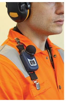
Noise dosimeters are small, body-mounted devices that collect individual exposure data, typically worn during an employee's entire shift. (photo courtesy Casella)
