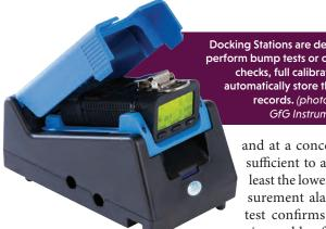
Docking Stations are designed to perform bump tests or calibration checks, full calibrations, and automatically store the testing records. (photo courtesy GfG Instrumentation)
