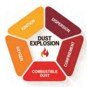
After an initial explosion or deflagration event, elastic rebound shockwaves occur, which cause more dust clouds. Secondary deflagrations and explosions are caused by the dust clouds jarred loose from the primary explosion. The explosion pentagon repeats itself until one of the five elements is no longer present. (Image courtesy Camfil APC)
