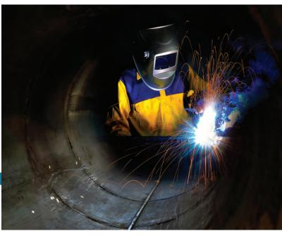
Local exhaust ventilation (LEV) is typically used when the task being performed produces high concentrations of toxic gases, vapors or fumes inside the workers' breathing area, such as confined space welding. (photo courtesy Adobe Stock)
