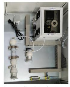
Shown here is a colorimetric analyzer in combination with a sample system for gas sampling in a harsh industrial environment. (photo courtesy DOD Technologies, Inc.)
