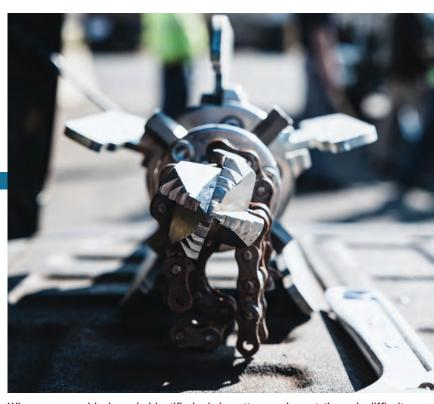
When a severe blockage is identified, chain-cutter nozzles cut through difficult obstructions and thick root masses. When high-pressure water enters the nozzle chamber, it is directed to spin the cutting chains at high velocity, with enough torque to avoid seizing. (photo courtesy KEG Technologies)
